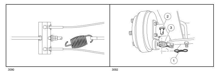
Figure 8-19 Disconnect Equalizer Spring
