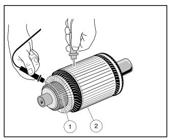
Figure 19-8 Armature Test
