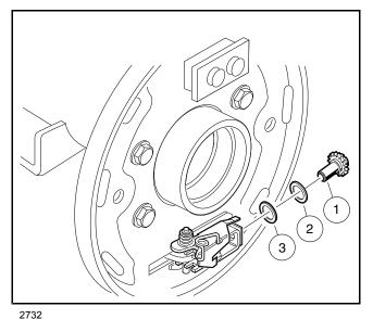
Figure 8-7 Remove Adjuster Wheel
