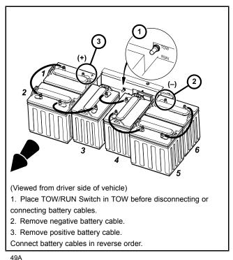
Figure 3-1 Battery Cable Removal
