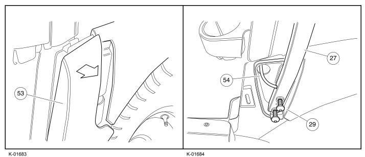
Figure 6-16 Pull Top of Floor Mat Retainer Outward
