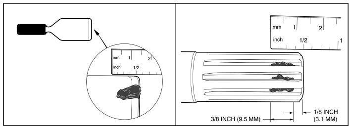
Figure 19-15 Grease on Putty Knife
