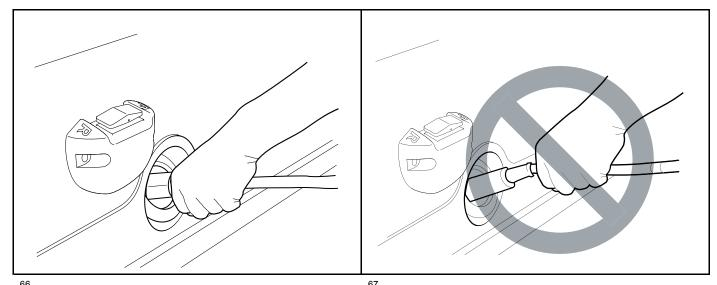
Figure 18-6 Correct Insertion of External Charger DC Plug
