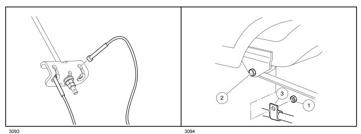
Figure 8-21 Disconnect Cables at Equalizer Bracket
