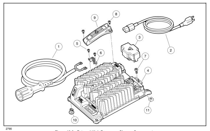
Figure 18-8 External High-Frequency Charger Components
