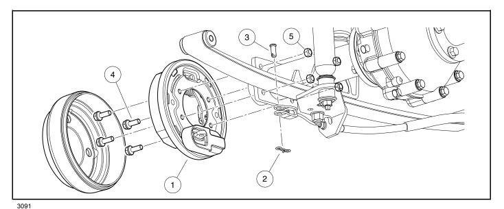
Figure 8-18 Brake Cluster Removal and Installation
