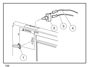
Figure 16-6 Tow/Run Switch
