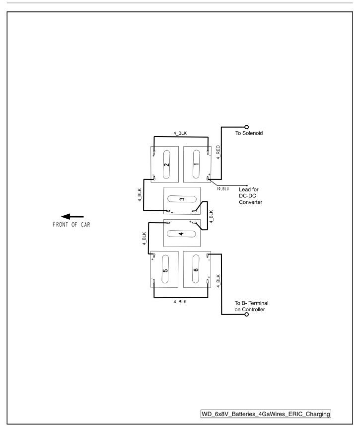
Figure 15-4 Battery Wiring Diagram – Precedent with ERIC Charging
