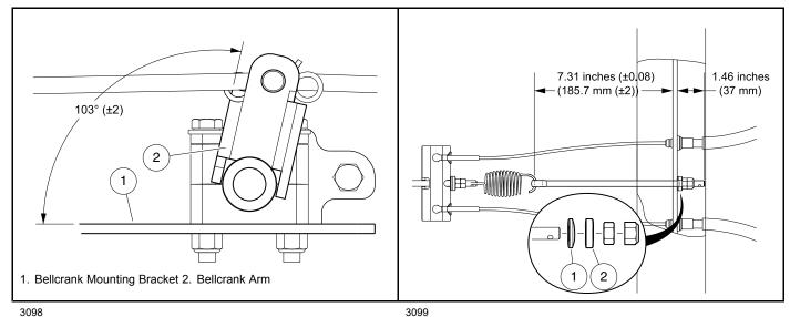
Figure 8-27 Proper Bellcrank Angle
