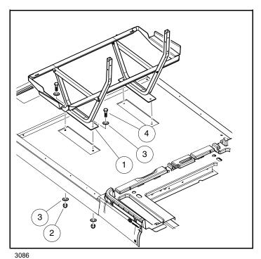
Figure 6-6 Remove Front Seat Frame
