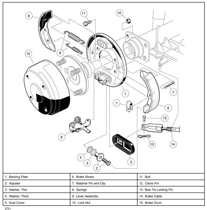
Figure 8-2 Self-Adjusting, Drum Brake Components
