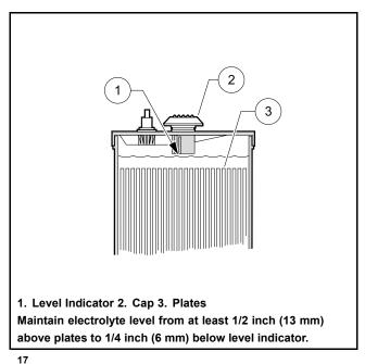
Figure 17-3 Battery Electrolyte Level
