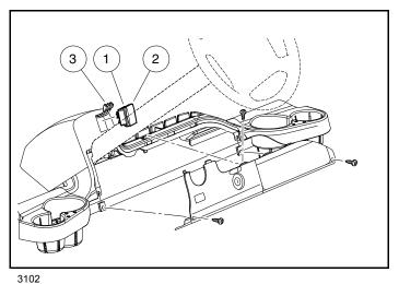
Figure 16-4 Forward/Reverse Rocker Switch
