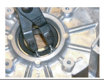
Figure 19-7 Retaining Ring Removal
