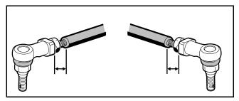
2064 Figure 9-9 Adjust Both Drag Links To An Equal Distance
