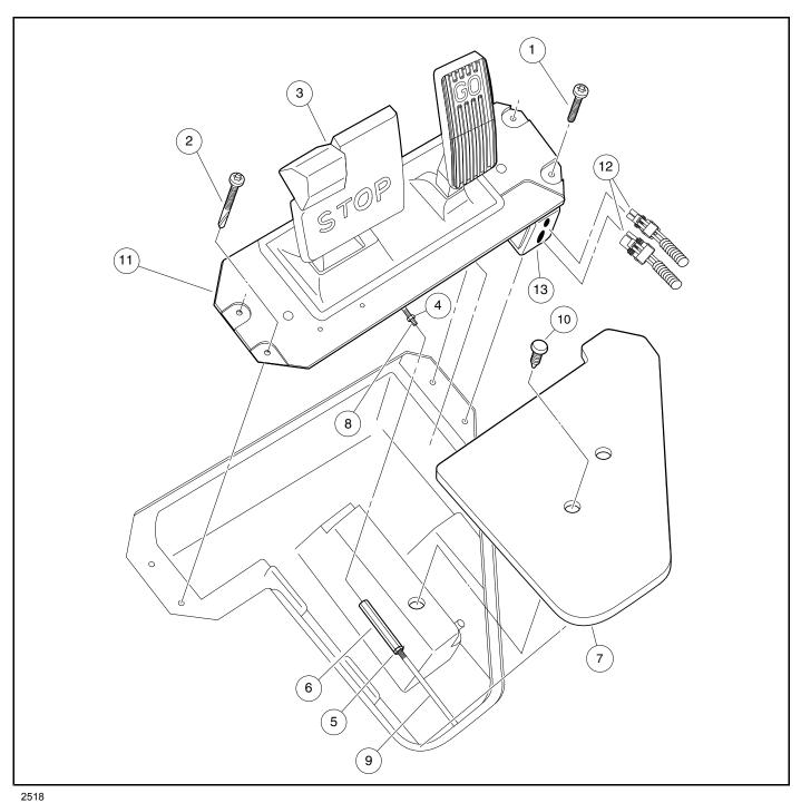
Figure 7-2 Pedal Group – Electric Vehicle
