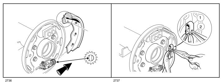
Figure 8-8 Install Adjuster Wheel, Trailing Shoe
