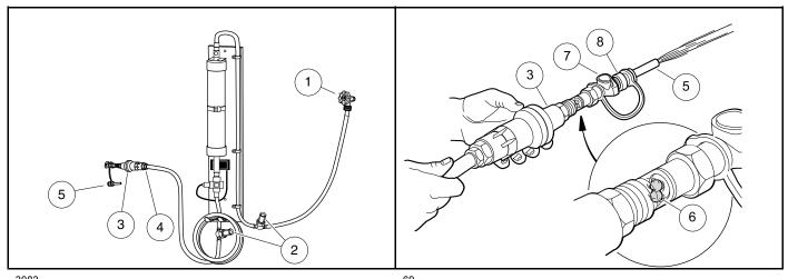
Figure 17-4 Connecting Hose with Filter to Water Source
