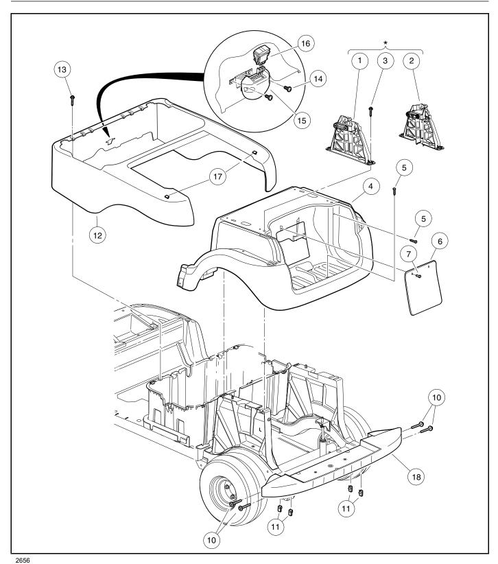
Figure 6-12 Rear Body Components
