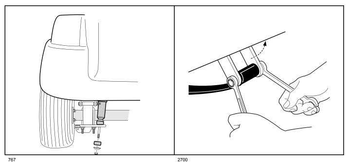
Figure 20-8 Disconnect Shocks
