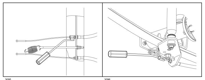
Figure 8-23 Release Brake Cables from Crossmember
