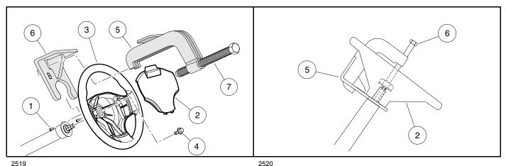
Figure 9-1 Steering Wheel Removal
