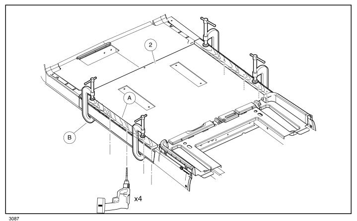
Figure 6-7 Drill Holes through New, Rear Floor Mat
