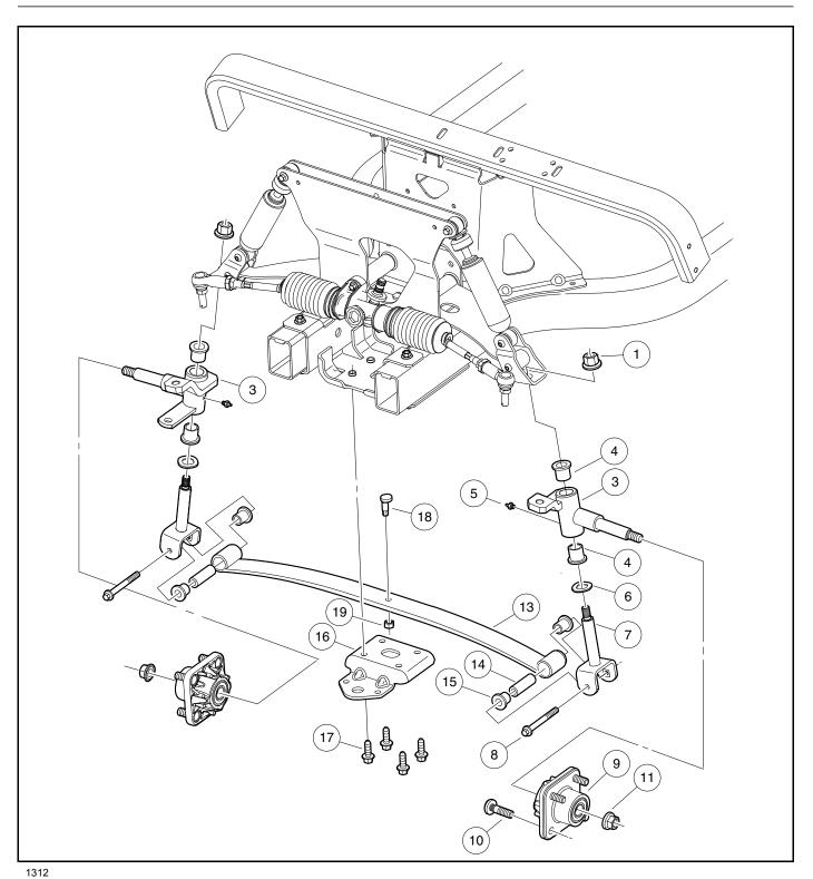
Figure 9-11 Lower Front Suspension Assembly
