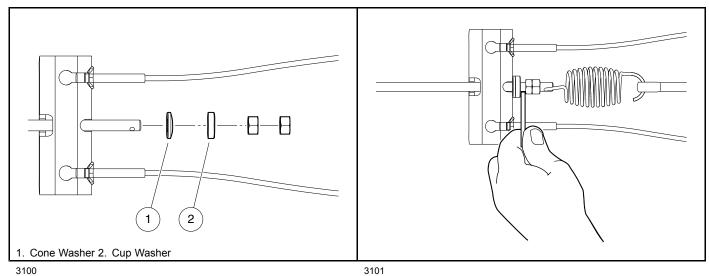
Figure 8-30 Cup and Cone Washer Orientation
