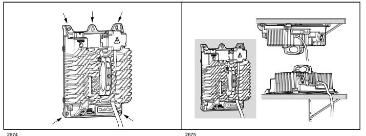
Figure 18-2 Charger Mounting Holes
