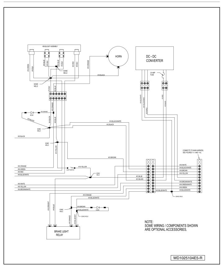
Figure 15-6 Precedent Electric Vehicle Accessory Wiring Diagram (Continued)
