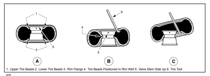
Figure 10-1 Tire Removal
