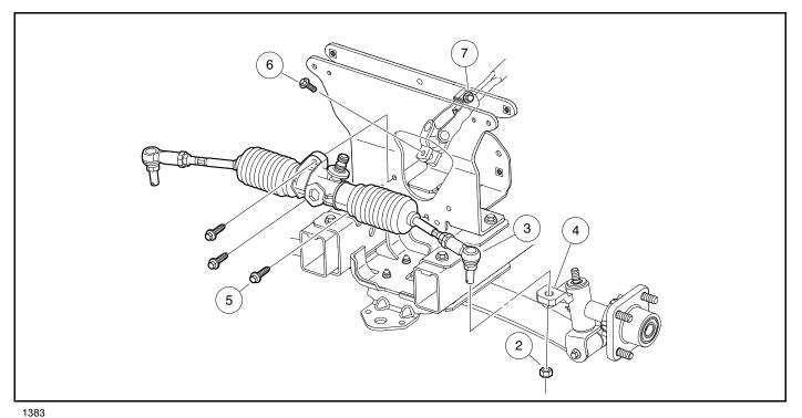
Figure 9-4 Rack and Pinion Removal
