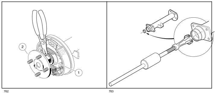
Figure 20-1 Remove Internal Retaining Ring
