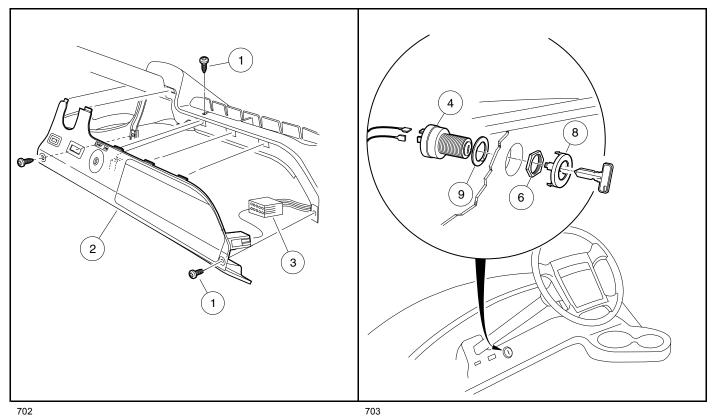
Figure 16-1 Instrument Panel Removal
