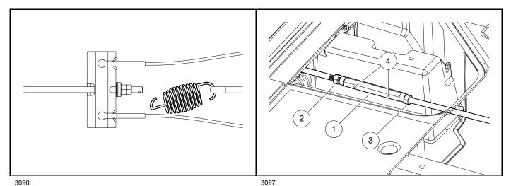
Figure 8-25 Disconnect Equalizer Spring
