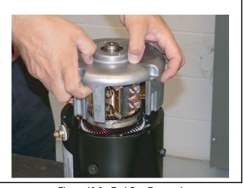
Figure 19-3 End Cap Removal
