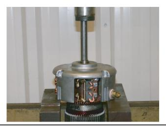
Figure 19-4 Brush Springs Positioning
