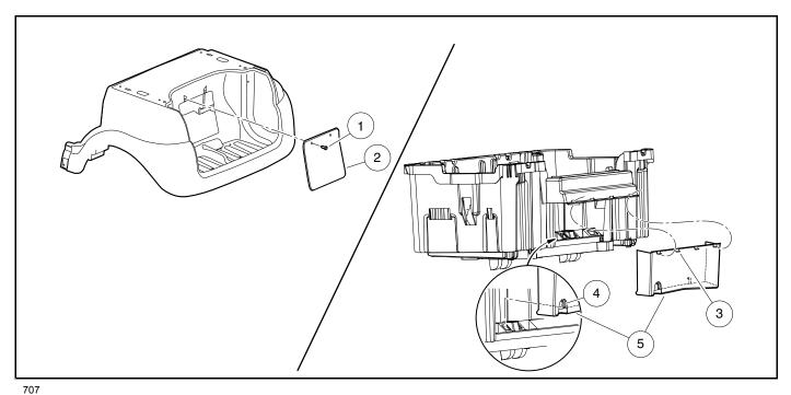
Figure 16-5 Access and Remove Electronics Module Cover
