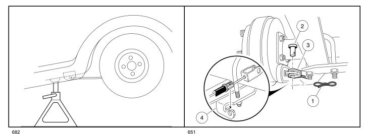
Figure 20-6 Vehicle Supported on Jack Stands
