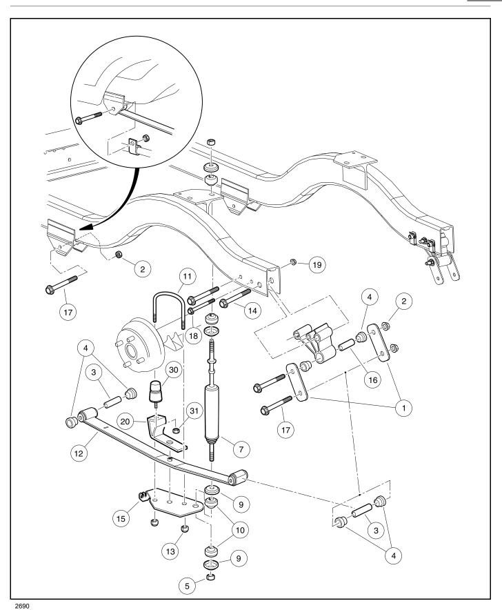
Figure 11-1 Rear Suspension Assembly and Mounting (Four-Passenger Vehicles)
