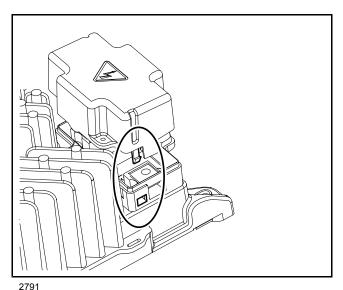
Figure 18-9 Terminal Block Cover Mounting Tabs
