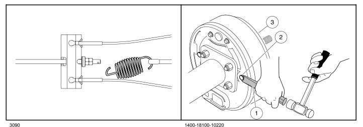
Figure 8-3 Disconnect Equalizer Spring
