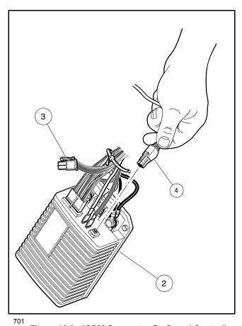
Figure 13-9 IQDM Connector On Speed Controller
