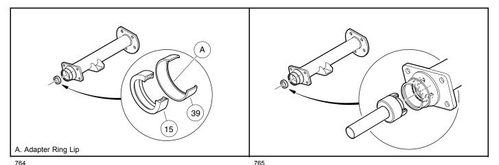
Figure 20-3 Axle Seal and Adapter Ring
