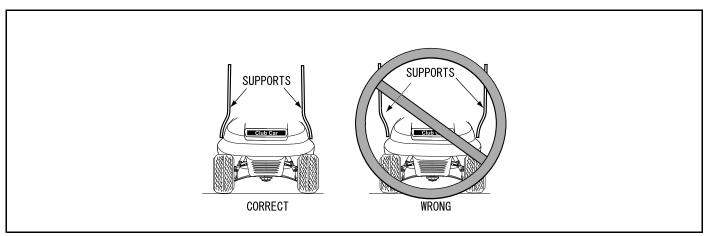
Figure 6-15 Properly Orient the Front Support Struts
