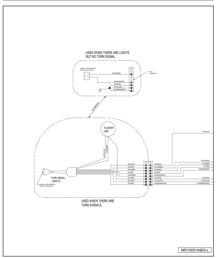
Figure 15-5 Precedent Electric Vehicle Accessory Wiring Diagram
