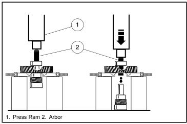
Figure 20-12 Intermediate Gear Assembly
