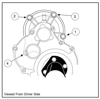
Figure 19-19 Motor Tightening Sequence
