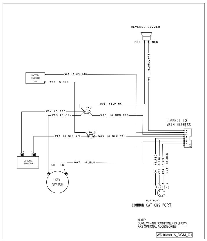
Figure 15-3 Instrument Panel Wiring Diagram – Precedent with ERIC Charging
