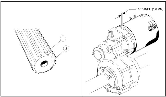
Figure 19-17 Clean Chamfer and Input Shaft End
