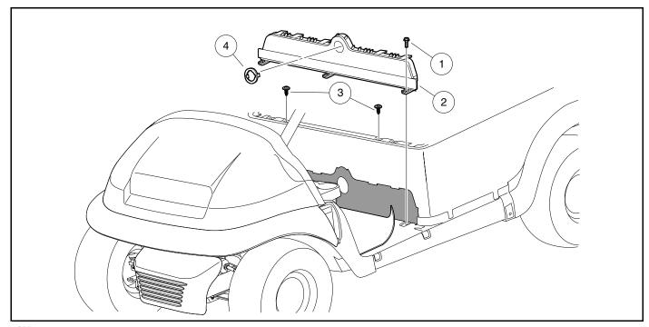
Figure 6-8 Kick Plate and Charger Receptacle Bezel
