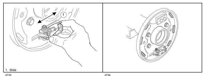
Figure 8-14 Lubricate Slide
