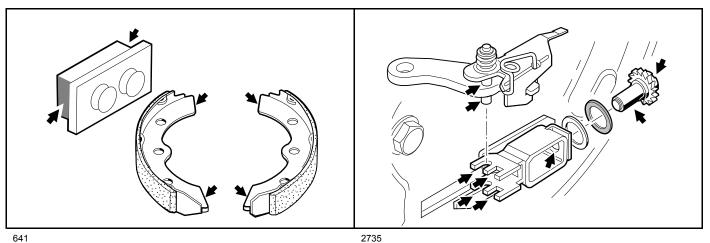
Figure 8-16 Apply Grease To Brake Shoes and Slots
