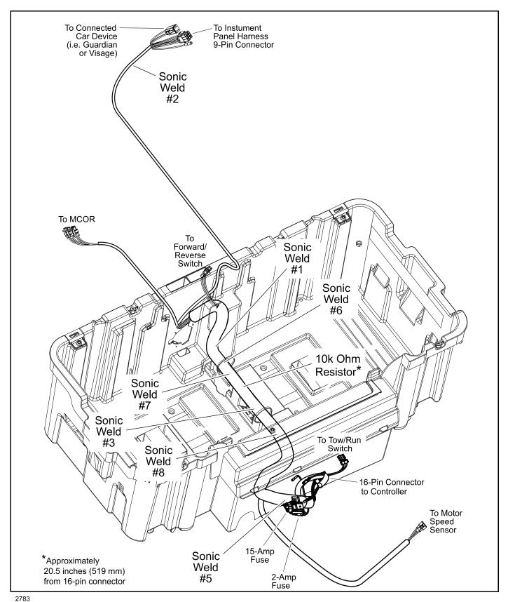
Figure 15-7 Sonic Weld and 10k Ohm Resistor Locations (Approximate)
