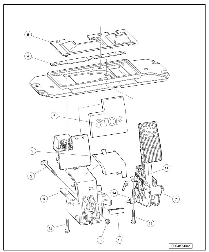
Figure 7-3 Accelerator Pedal Assembly and Brake Pedal Assembly
