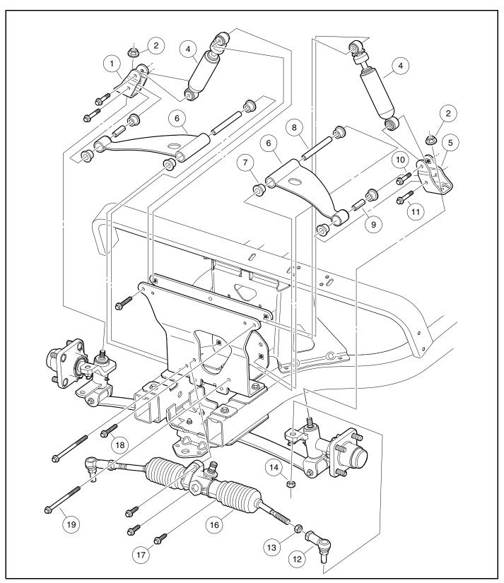
Figure 9-10 Upper Front Suspension Assembly
