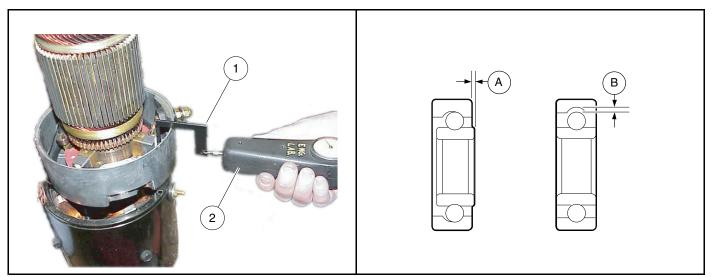
Figure 19-9 Brush Spring Tension Test
