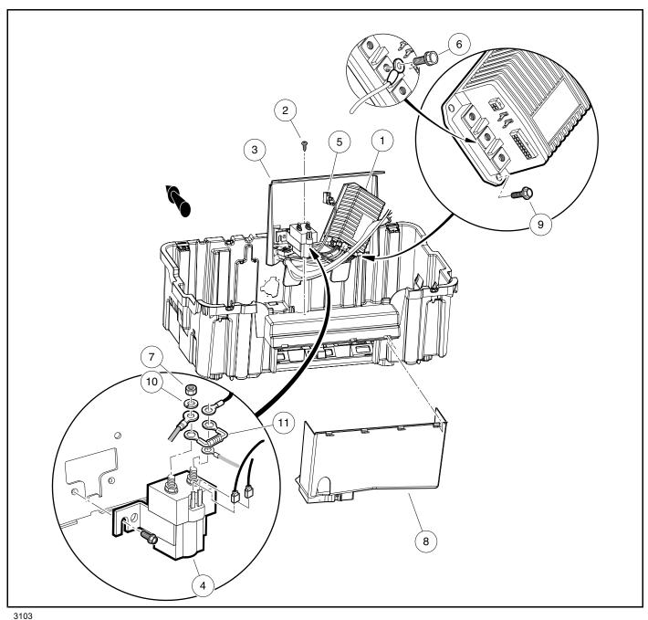
Figure 16-8 Controller and Solenoid Removal
