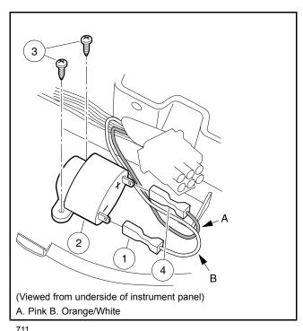
Figure 16-7 Reverse Buzzer
